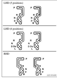
While depressing the brake pedal, move the selector lever through the gate.
