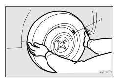
7. Temporarily tighten the wheel nuts by hand until the tapered parts of the wheel nuts make light contact with the seats of the wheel holes and the wheel is not loose.
