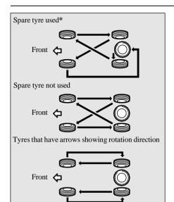
\*: If the spare tyre differs from the normal tyre, do not perform tyre rotation using a spare tyre.
