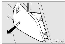
4. Turn the socket anticlockwise to remove it.
