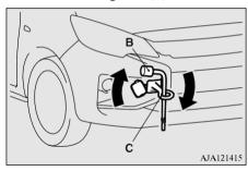
4. Secure the tow rope to the front towing hook.
