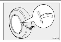
2. With the cover raised a little, pry it off completely using the jack bar. Insert the jack bar under the cover, and move it around the circumference, prying the cover away from the wheel little by little as you move the bar around.
